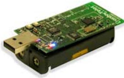
Figure 1: The Telos WSN node with embedded sensors and in board antenna presented here with its packaging for 2 AA batteries. The overall packaging box size is 20 \times 60 \times 35\text{mm} .
