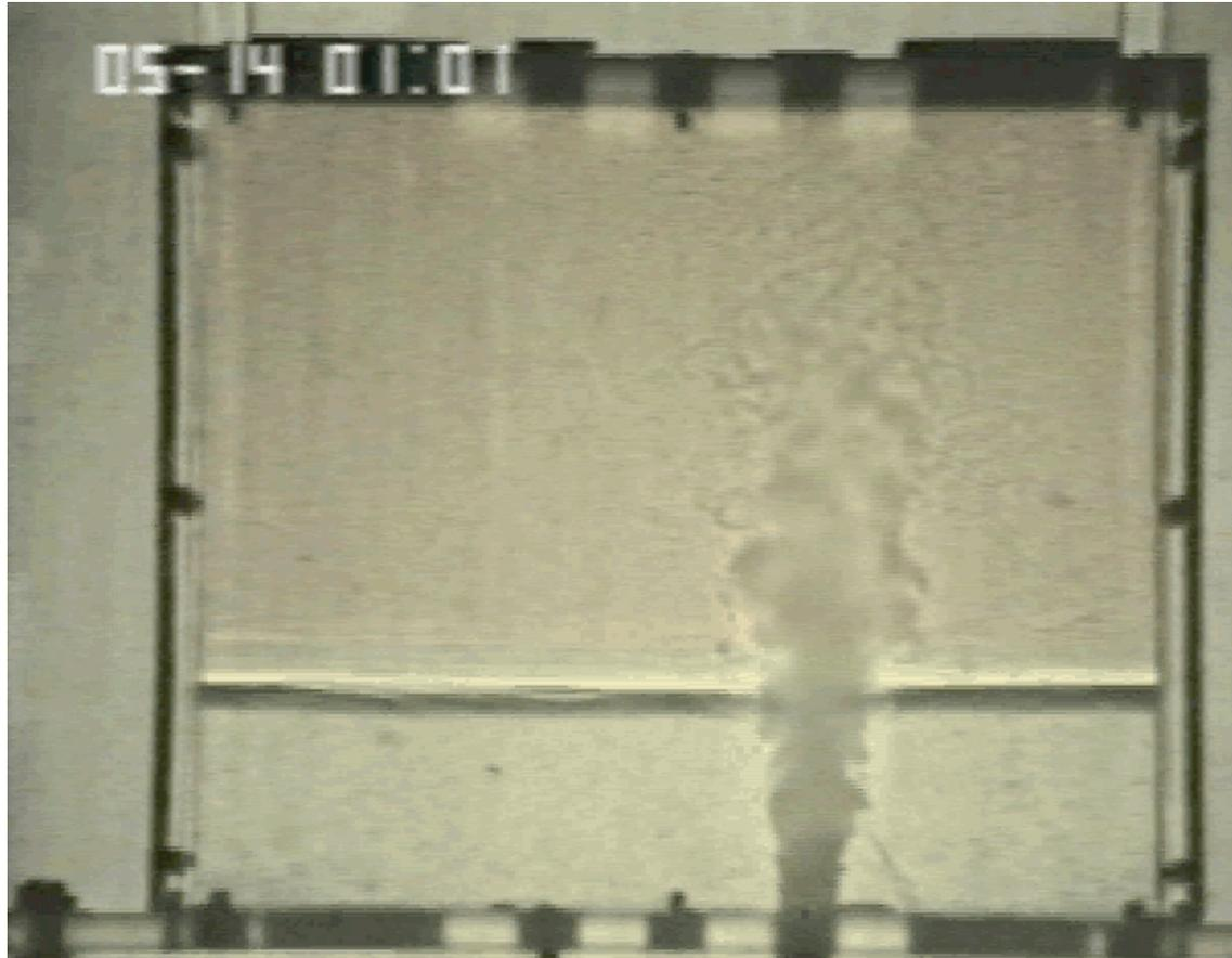
Steady state consists of two uniform layers of different temperatures
