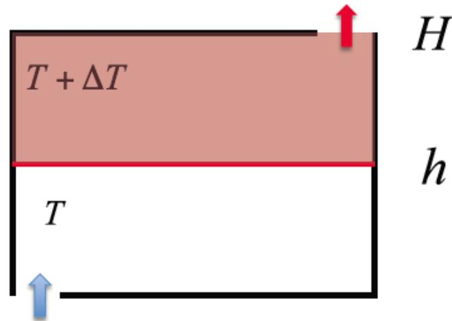
The pressure difference associated with the hot upper layer across the upper opening  $A_U$
