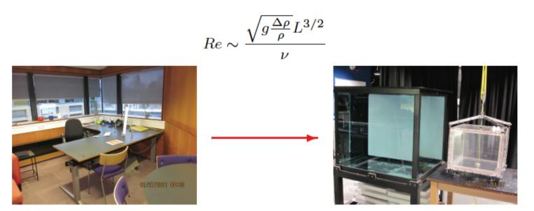
In a typical model  $L_{lab} \sim \frac{1}{20} L_{build}$  so unless we change the properties of the fluid  $\Rightarrow Re_{lab} \sim \frac{1}{100} Re_{build}$
