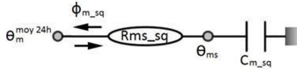
Figure 4: Secondary RC network for sequential inertia calculations
