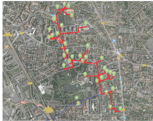
Figure 1: Layout of Blagnac heating network
