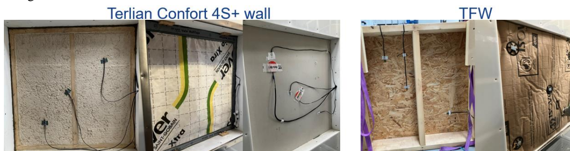
Figure 2 : picture of the two prototypes mounting and insertion in the bi-climatic chamber frame.
