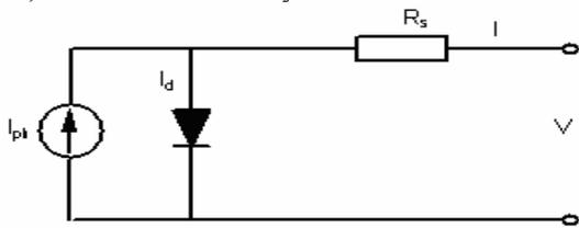
Figure 6: Equivalent circuit of a four-parameter PV model.
