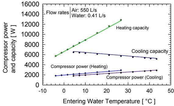
Figure 4: Heat pump performance data.
