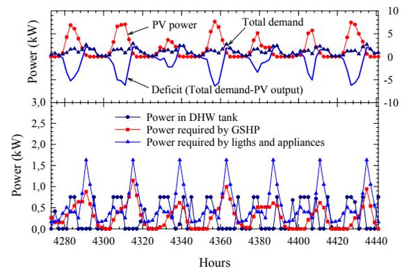
Figure 10: Power requirements and production for a typical summer week.
