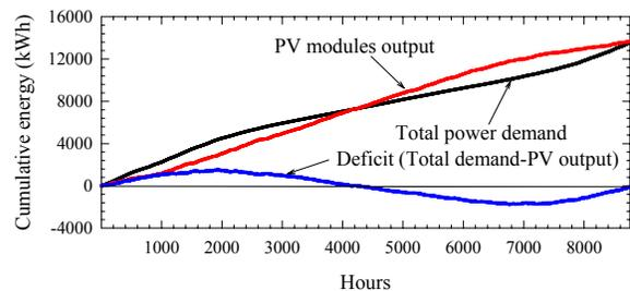
Figure 11: Cumulative energy requirements and production.
