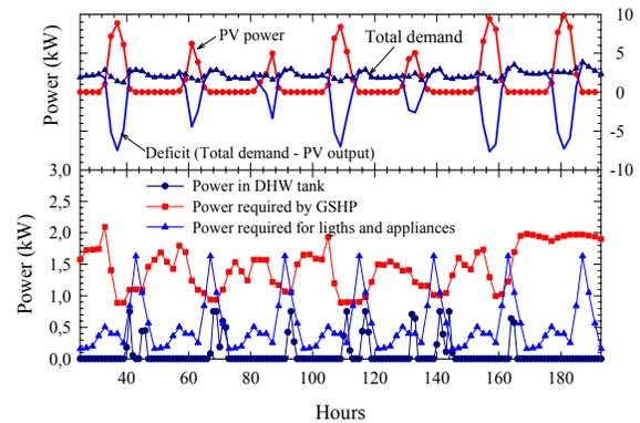
Figure 9: Power requirements and production for a typical winter week.
