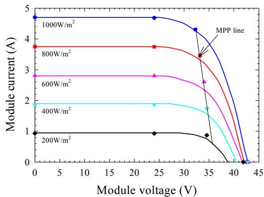
Figure 7: I-V curves for a cell temperature of 25°C and different irradiance levels. Manufacturer's data (curves) and results from TYPE 94 (data points).
