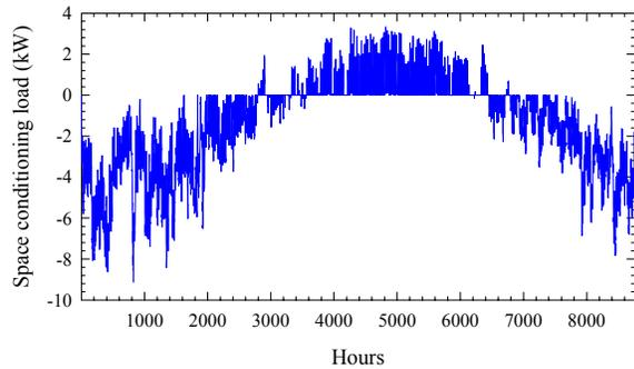
Figure 8: Hourly space heating and cooling loads.
