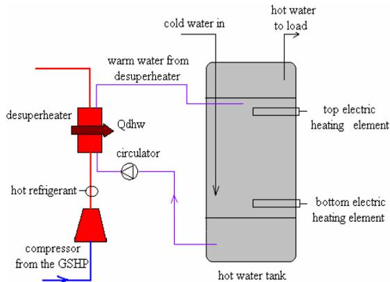
Figure 5: Domestic hot water pre-heating using a desuperheater.
