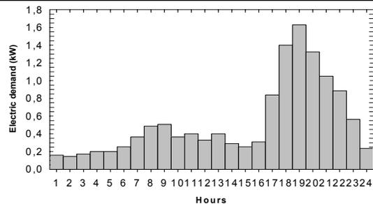
Figure 2: Lights and appliances electrical load profile.
